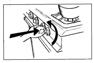
The flame should be adjusted so it does not extend beyond the edge of the cooking utensil. This improves your cooking efficiency, insures your personal safety and prevents damage to any cabinets above the range.
