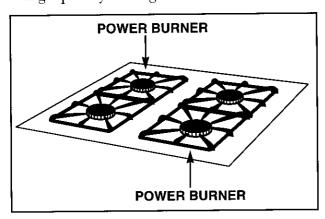
A properly adjusted burner with clean ports will light within a few seconds. If using natural gas, the flame will be blue with a deeper blue inner core; there should be no trace of yellow in the flame (this indicates an improper mixture of air/gas which wastes fuel and should be adjusted by a service technician) With LP gas, some yellow tips on the flames are acceptable. This is normal and adjustment is not necessary.
