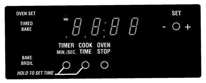
The electronic clock on your Maytag range is used for the time-of-day clock, timer and delay start functions. At the end of an operation, consecutive beeps will sound.
