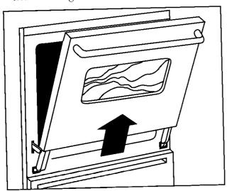
CAUTION: The hinge arms are spring mounted and will slam shut against the range if accidentally hit. Never place your hand or fingers between the hinges and the front oven frame. You could be injured if the hinge snaps back.
