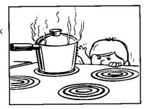
children. To minimize burns, ignition of flammable materials and spillage due to unintentional contact with the utensil, do not extend handles over the adjacent surface burners.
