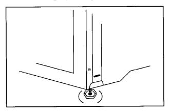
warning: To reduce the risk of accidental tipping of the range, it must be secured by a properly installed anti-tip device. To check if the device is installed properly, use a flashlight and look underneath the range to see that one of the rear leveling legs is engaged in the bracket slot. The anti-tip device secures the rear leveling leg to the floor, if properly engaged.
